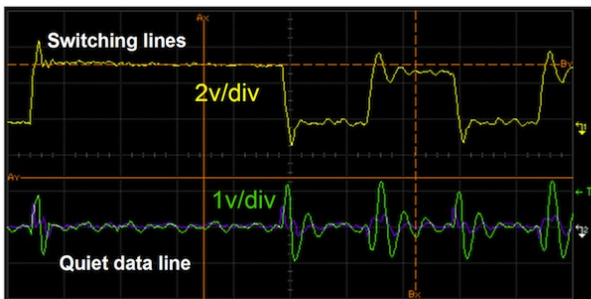
Figure 1 Example of the measured ground bounce on a quiet line.
