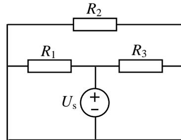
DATOS:  $R_1 = 1 \Omega$ ,  $R_2 = 2 \Omega$ ,  $R_3 = 3 \Omega$ ,  $U_s = 12 \text{ V}$ .
