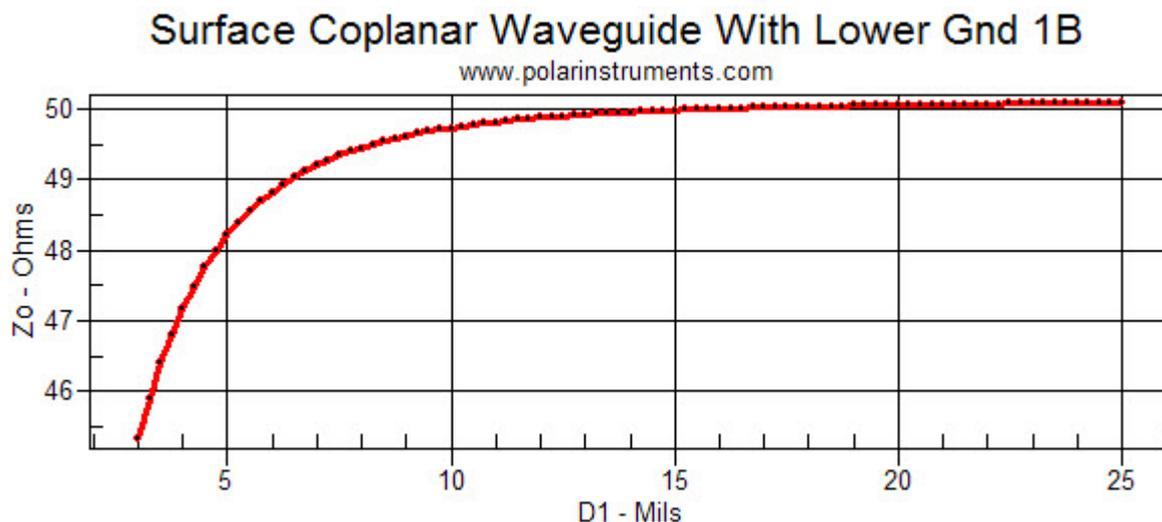
Note the vertical axis scale is 1Ω per division. When the spacing to the adjacent metal is farther than three line widths - 15 mils - there is no impact.
