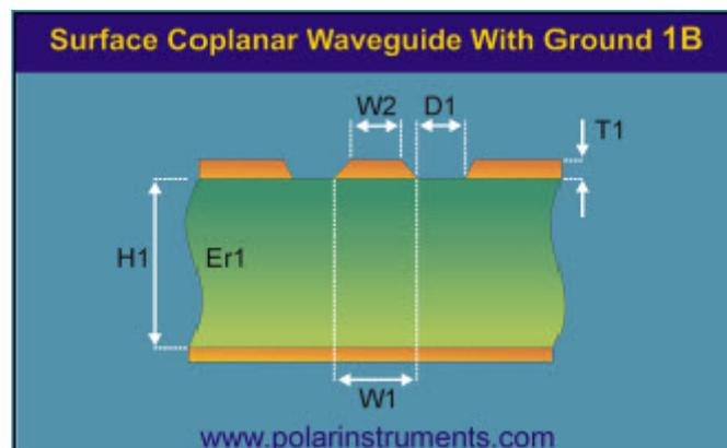
The conductors on either side of the signal line on the top layer are connected to the return path on the bottom.
