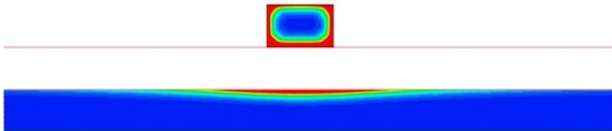
**Figure 1. Current density in a microstrip at 100 MHz. Blue means no current, red means a lot of current. Simulated with ANSYS SI2D.**
