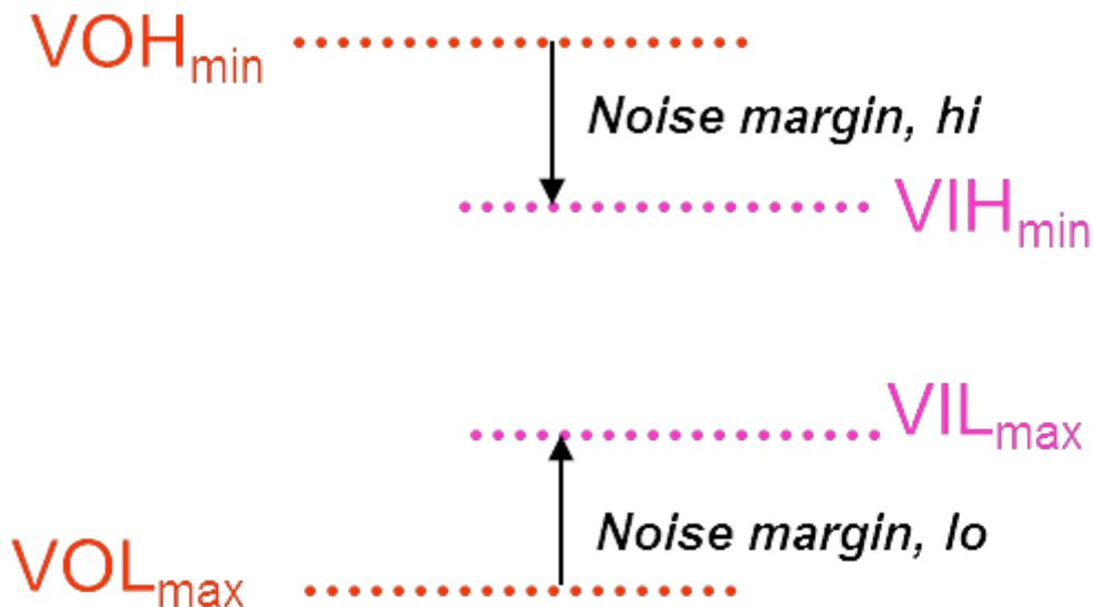
The difference between the worst voltage from the Tx and the worst at the Rx is the amount of “wobble” room available. It is the amount of noise that can be tolerated before the Rx signal exceeds the limits to an accurately received 1 or 0. We call this difference the “noise margin.”
