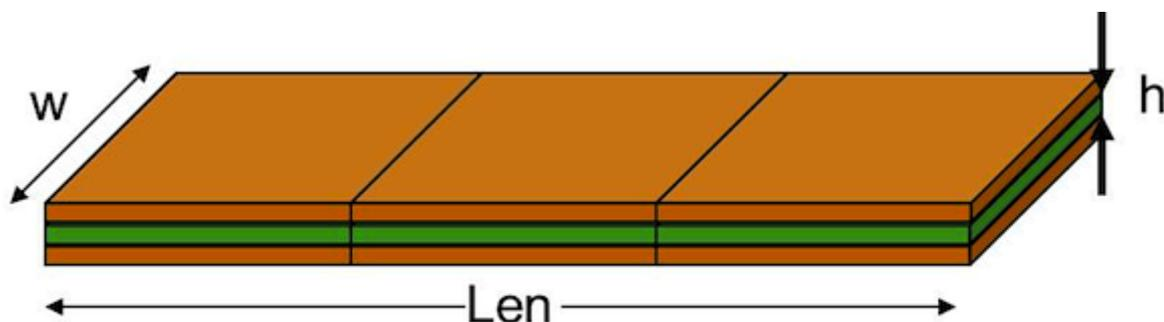
This assumes the current flow is uniform from the left edge of one trace, down the long length, connecting to the other trace at the right end, and flowing back on the other trace to its left edge.
